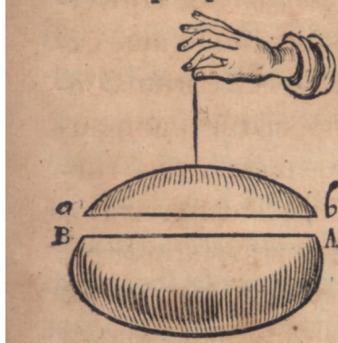
Figure 14. A magnet divided along the axis between the poles A and B. Upper part held by a hand using a thread to allow free rotation. Poles are labeled (a, b, A, B). The diagram is schematic but includes a performative feature (hand) and adds hatching to the egg-shaped magnet. (Woodcut print on paper.) From Principia philosophiae (p. 279) by R. Descartes, 1644, Amsterdam, The Netherlands: Apud Ludovicum Elzevirium (Berlin, Max-Planck-Institut für Wissenschaftsgeschichte, Bibliothek, Rara D445pr).
