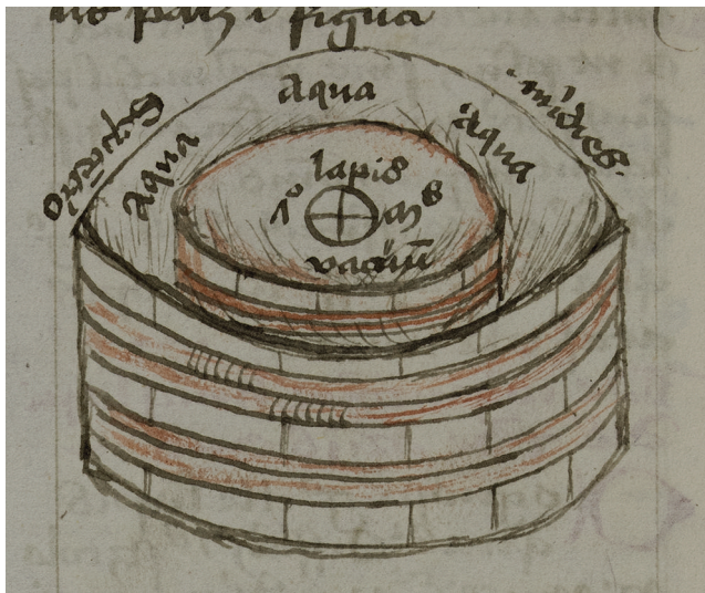
Figure 6. Vessel filled with water in which a smaller vessel floats, carrying a magnet. Water ( aqua ), cardinal directions ( septentrio , meridies ; labeled both for the vessel and for the magnet), and the magnet ( lapis ) in the center are labeled. The axis and equator of the magnet are indicated diagrammatically with lines. Visually, the drawing of the vessel has features that make it look naturalistic (for example, perspective and slight hatching), and it even depicts the probably wooden staves bound by hoops, distinguished by color. Abstract and more naturalistic features are combined in this hybrid diagram. (Illustration inserted into the text by the scribe, ink on paper.) From Rome, Biblioteca Apostolica Vaticana, Pal. lat. 1340 (14th century), fol. 31v.
